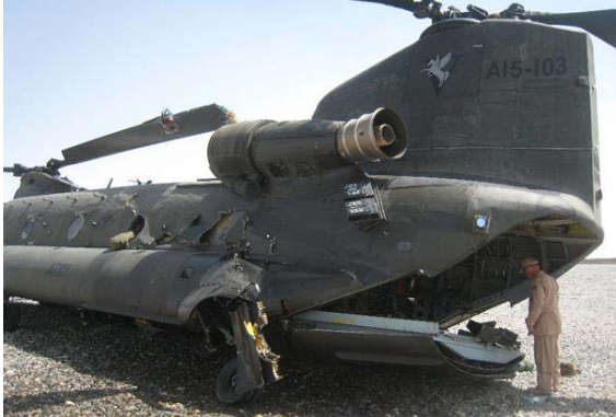
A15-103 in situ, emphasizing failed landing gear (Photo by C Kerr)
