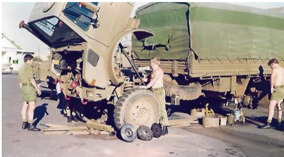
FRG 301 Fd Wksp undertaking repairs to a Unimog on Exercise K89
