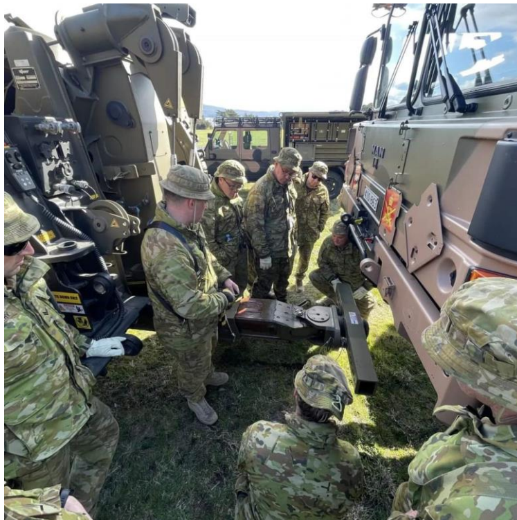
CPL A. Warsing instructs on the correct hook up procedure on the 42M medium recovery vehicle.
